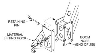
Figure 8-2. Material Lifting Hook Installation
